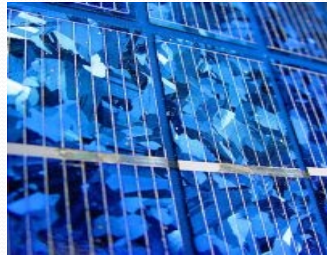
Visible crystal grain in poly-Si
