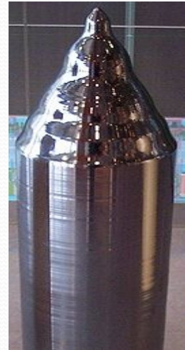
Si boule for the production of wafers.
